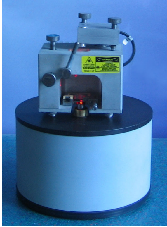
Figure 1.2. Mechanics of FemtoScan microscope.
